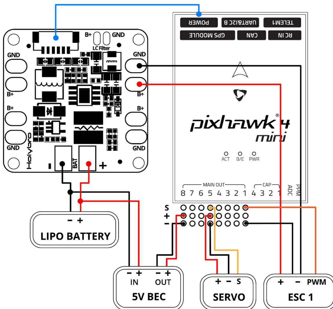
Note: The image above only shows the connection of a single ESC and a single servo. Connect the remaining ESCs and servos similarly. Refer to Airframe Reference ([https://docs.px4.io/en/airframes/airframe\\_reference.html](https://docs.px4.io/en/airframes/airframe_reference.html)) to connect ESCs to **MAIN OUT** in the correct order for your airframe configuration.
