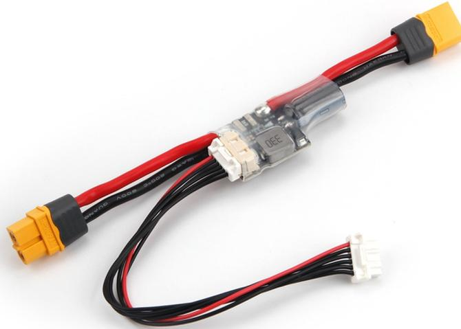
PM02D provides regulated power supply for your Pixhawk<sup>®</sup> 5X from the battery, as well as current consumption and battery voltage measurements, all through a 6pin cable. The on-board switching regulator outputs 5.2V and a maximum of 3A from LiPo batteries up to 6S. The Power Module comes completely assembled with XT60 connectors, wrapped in shrink tubing for physical damage protection.
